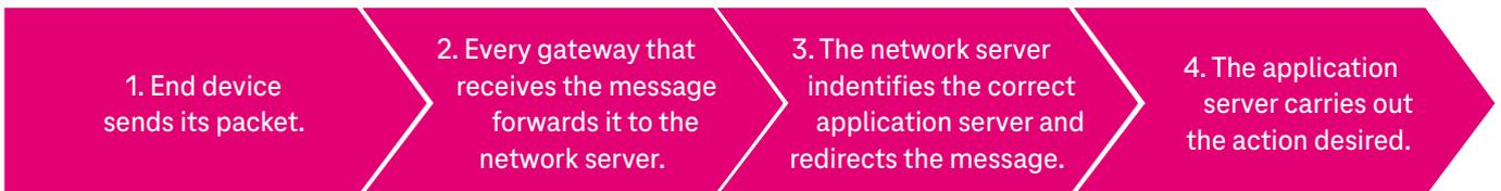
Figure 3: LoRaWAN v1.0 architecture [4]
