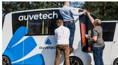
Auve Tech mounting PGM on a driverless shuttle
