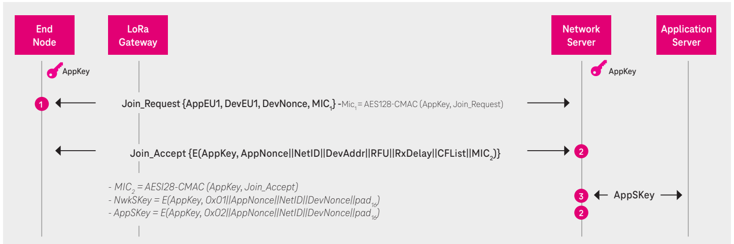
Figure 4: OTAA registration process of a LoRaWAN device [9]
