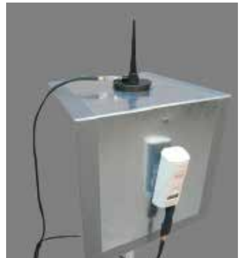
Figure 1: Measurement setup showing the scanner antenna (on top) and the housing containing the antenna feeding the Quectel BG96 module
